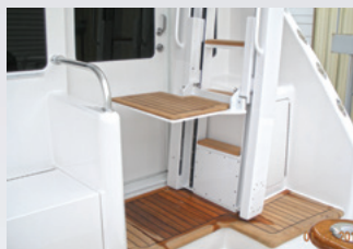
Integrated elevator & bridge ladder
