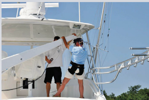
Bluewater staff demonstrate the hinged belly band and custom davit designed to lift Jones and his motorized chair
