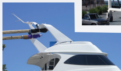
Bluewater Yacht Yard staff finishing the skybridge and custom fabricated radar arch on the Viking 76EB
