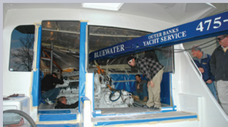
One of the Bloom's prior boats, the 68EB, undergoing a repower in 2010
